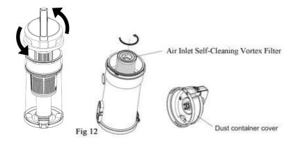
**NOTE:** The Prolux Self-Cleaning Vortex filter only needs to be cleaned when the entire surface of the filter becomes dirty. Due to its highly efficient design the Self-Cleaning Vortex filter is three times more efficient than standard filters and will have the same amount of airflow whether it's dirty or clean. The entire surface of the filter will have to be covered in debris before the performance of the vacuum is affected, and the filter needs to be cleaned.
