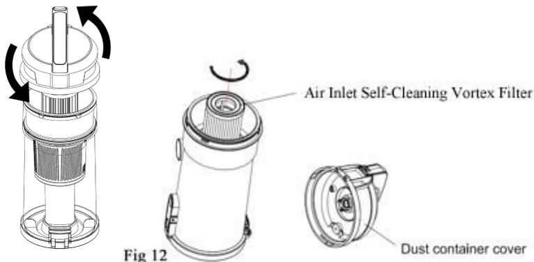
**NOTE:** The Prolux Self-Cleaning Vortex filter only needs to be cleaned when the entire surface of the filter becomes dirty. Due to its highly efficient design the Self-Cleaning Vortex filter is three times more efficient than standard filters and will have the same amount of airflow whether it's dirty or clean. The entire surface of the filter will have to be covered in debris before the performance of the vacuum is affected, and the filter needs to be cleaned.
