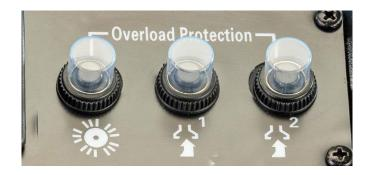
This machine is equipped with resettable circuit breakers which protect the electronic components. In the event the circuit breaker is tripped during use, turn the machine off completely and unplug it from power. Wait for the machine to cool if any parts feel or appear overheated.
